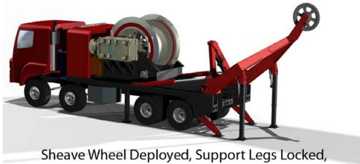
Sheave Wheel Deployed, Support Legs Locked,
